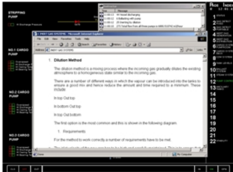
Example of main display showing additional information about the Dilution method of inerting tanks accessed via the short operator message.
